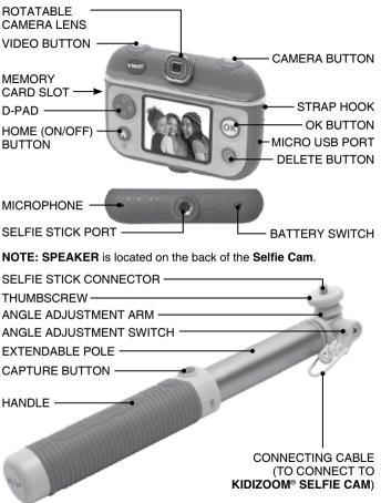
**NOTE:** The **THUMBSCREW** on the Selfie Stick adjusts the length of the **SELFIE STICK CONNECTOR** so you can securely mount the camera facing in any direction. To prevent damaging the **Selfie Cam**, do not detach the **THUMBSCREW**.
